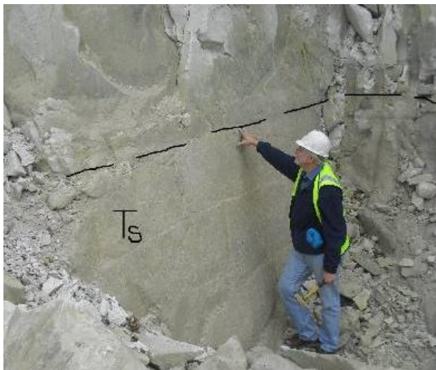
Photo above: Dr. Oates points out the top of the more massive bedded Totternhoe Stone.
