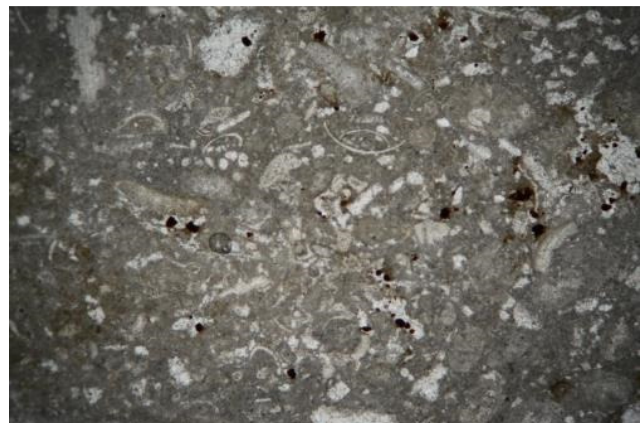
Thin-section image. Coombs Quarry. Bioclastic rich limestone with common disarticulated ostracod valves. Plane polarised light, x 50. Field of view 5 mm.
