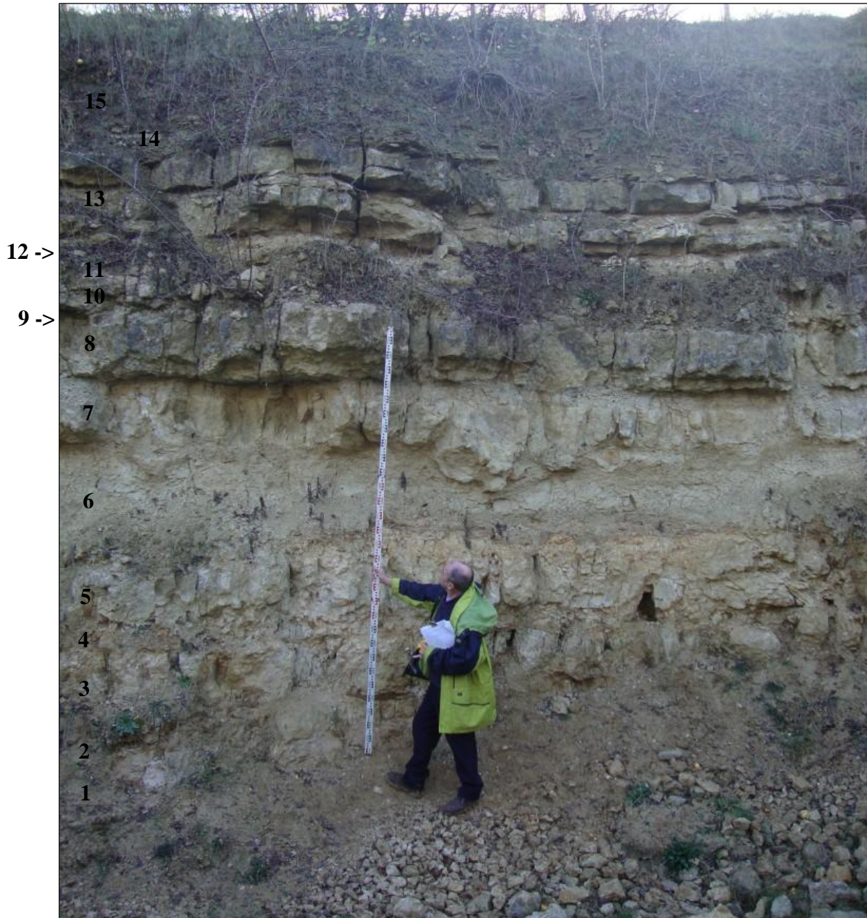
Figure 2 The south face Coombs Quarry showing the White Limestone beds (the Forest Marble Formation is at the top of the section obscured with vegetation and slip). Note that the hardness and hence weathering of the beds, does not match major lithological breaks, and reflects differences in cementation.
